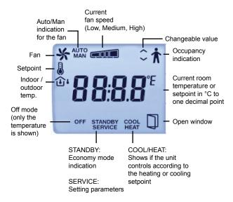
The display is handled using the buttons on the controller:
