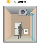
In 4-pipe installations, there are two separate pipe systems for heating and cooling with separate valves. The controller uses two outputs for control of heating and cooling in sequence.
