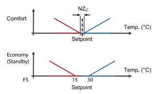
The above schematic drawings of the control principle show the corresponding requirement of the controller function. This requirement is recalculated by the controller to a value for the actuator output, depending on the selected output function.
