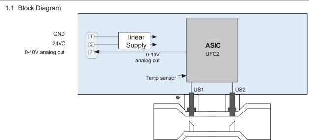
The Ultrasonic Flow Sensor is constructed with a flow tube , two ultrasound transmitters and an electronic device. The electronic device is based on Application-Specific Integrated Circuit (ASIC) to perform the ultrasonic time-of-flight measurement between the two ultrasound transmitters. A temperature sensor is placed in the flow tube to compensate temperature effects.
